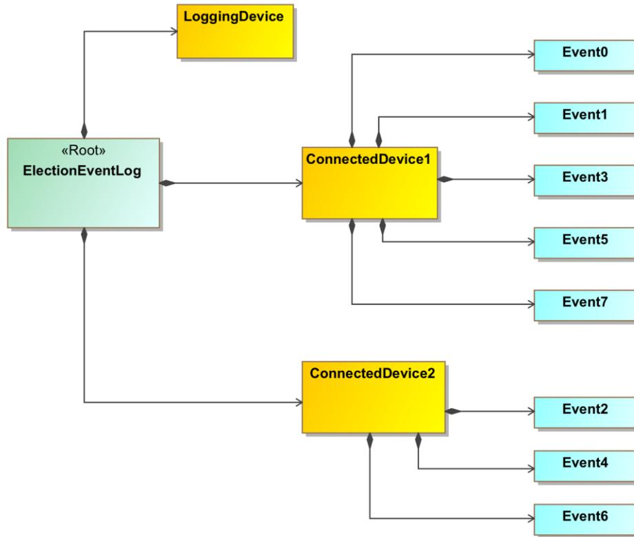
Figure 4 - Third use case for a logging device connected to event generating devices
